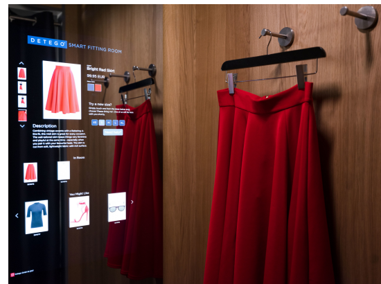
Figure 1: Smart Fitting Room . RFID-enabled smart fitting rooms bridge the gap between online and brick-and-mortar stores by providing features such as additional product information and product recommendations.
